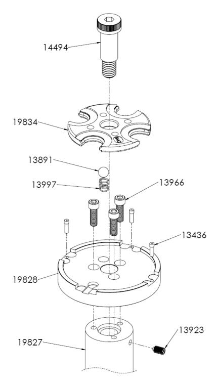
**NOTE:** Before attempting to remove the shellplate bolt (PN: 14494) be sure that the shellplate bolt set screw (PN: 13923) is removed.
