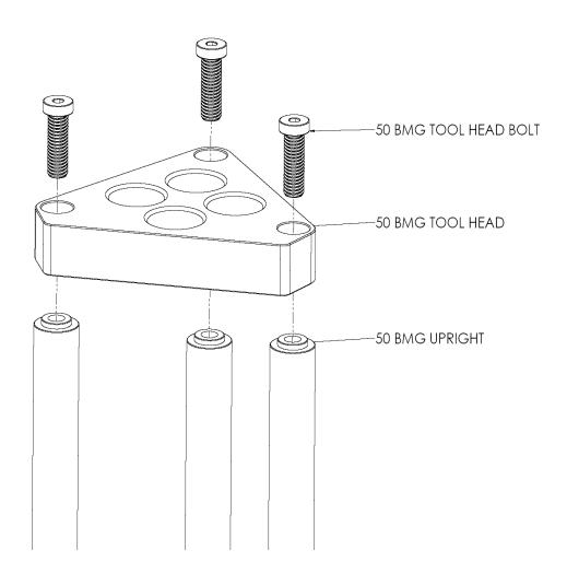
Changing the Toolhead will require the removal of the three Toolhead Bolts, then lift the Toolhead straight up and off of the three Uprights. To replace the Toolhead simply place it back on the three Uprights aligning the pockets on the bottom of the Toolhead and the steps on the top of the Uprights. It may be necessary to loosen the lower right front Upright mounting bolt to get the Toolhead to seat fully. Replace and tighten the Toolhead Bolts (35-40 ft/lbs torque).
