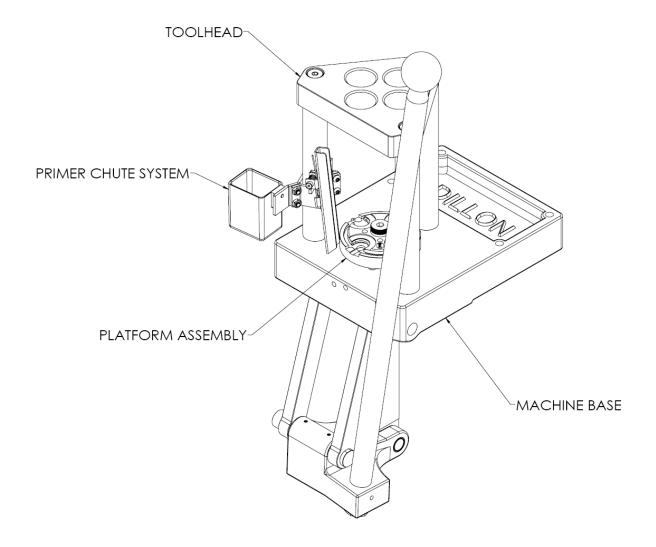
This is the basic layout of the machine. Noted above are the primary sub assemblies which are detailed in the following pages. Once your machine is mounted you will need to install the "Spent Primer Catch System" on to your machine. Start by removing the four mounting screws and nuts from the assembly (Part# 29009 and 16340). Assemble it onto the front left side post on the machine as shown in the diagrams below.
